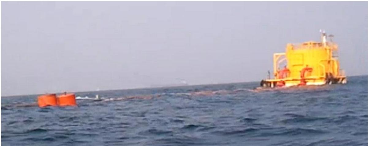
**Figure 3.10** Turret Buoy with Floating Hoses
