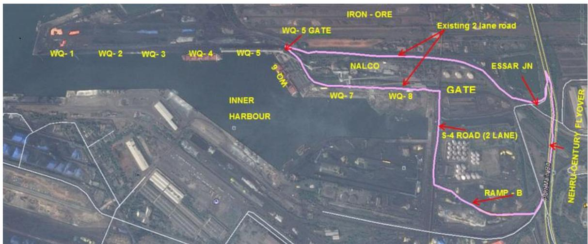
**Figure 8.5** Connectivity of WQ Berths
