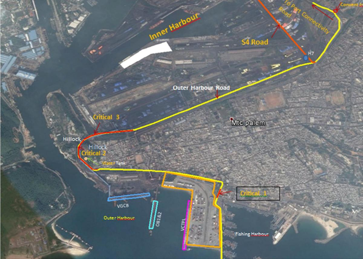
**Figure 8.8 Outer Harbour Road with Critical Locations for Widening (4 Lane Road Proposal)**
