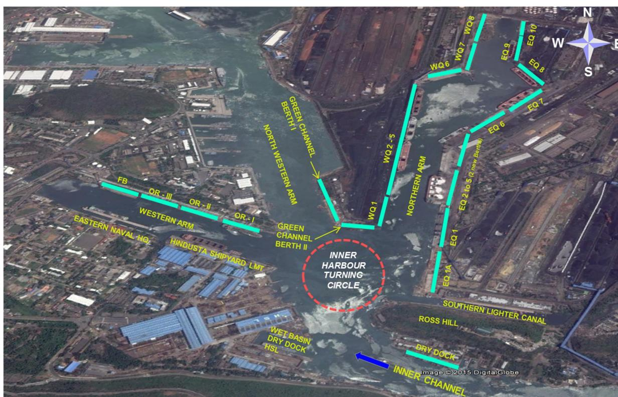
**Figure 10.4 Layout Plan of Inner Harbour 2030**
