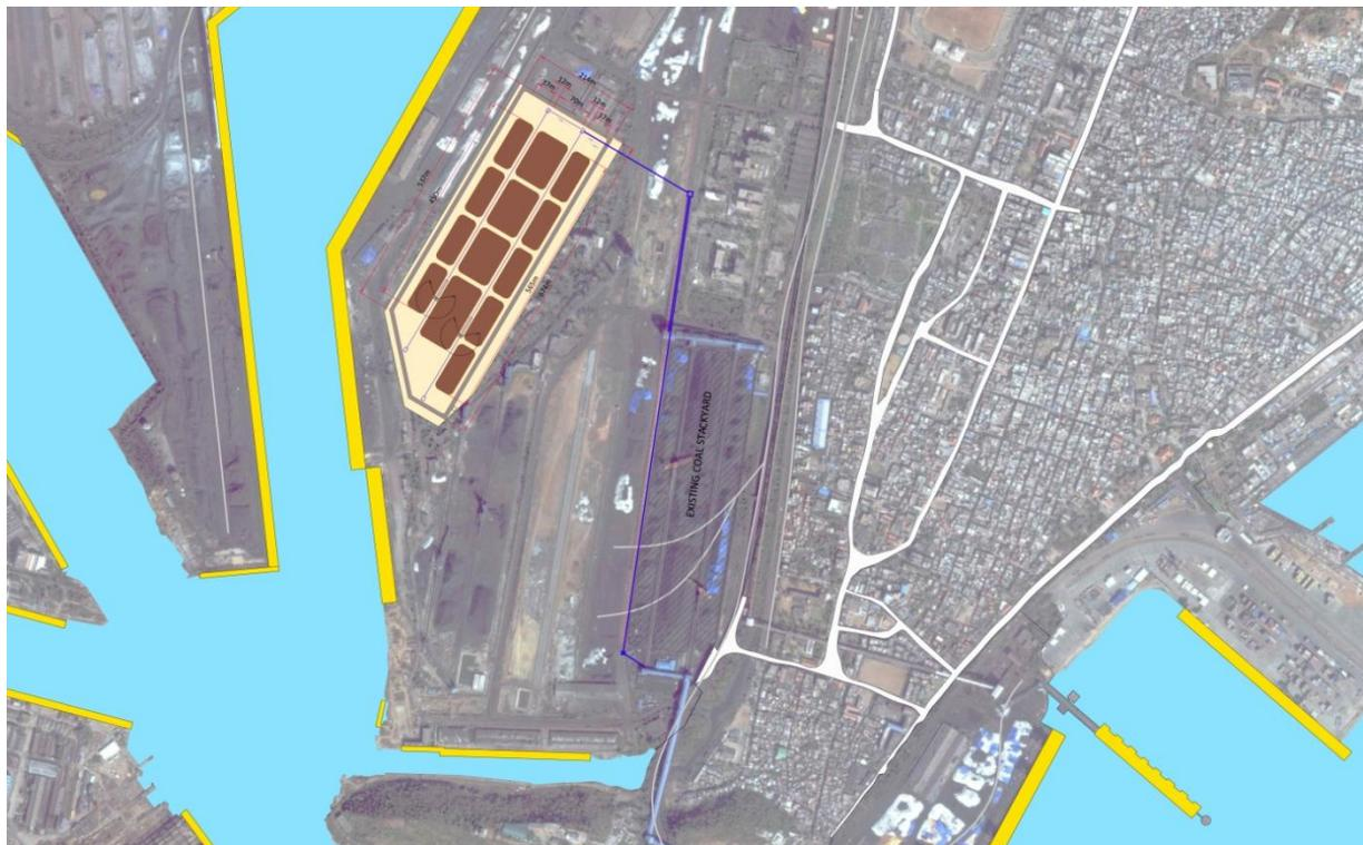
**Figure 7.2 Additional Stackyard – Location, Layout & Route of Conveyors**
