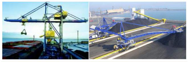
Figure 143: Some examples of coal terminal equipment. Gantry crane (left) and stacker/reclaimer (right)
