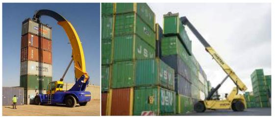
Figure 141: Two different types of reach stackers (RS)
