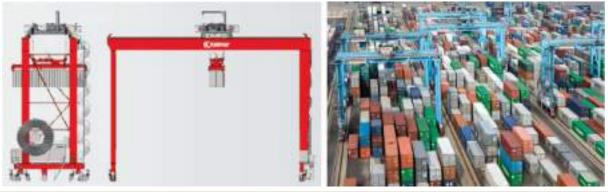
Figure 140: Scheme and twin A-RMGs in an automated container yard
