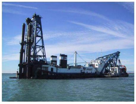
Figure 132: Cutter Suction Dredger
