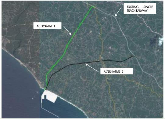
Figure 13. Alternatives 1 (green) and 2 (black) for rail connectivity
