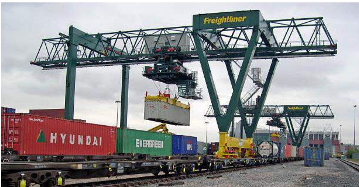
Figure 142: Rail yard with Rail Mounted Gantry cranes
