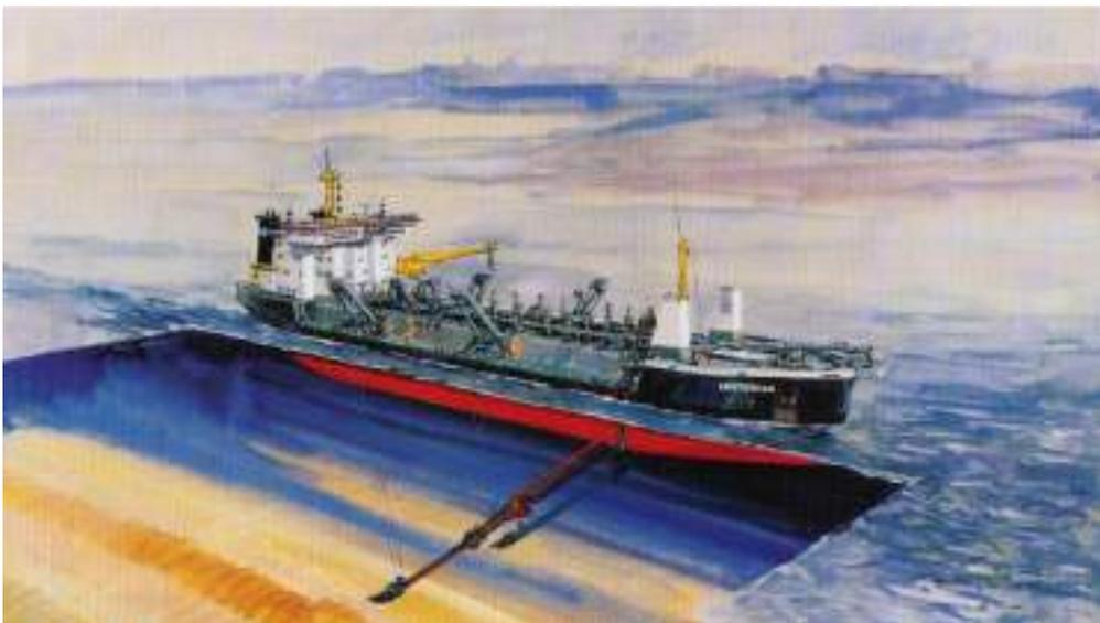
Figure 133: Trailing Hopper Suction Dredger
