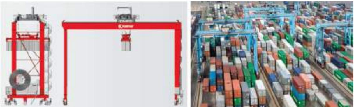
Figure 140: Scheme and twin A-RMGs in an automated container yard
