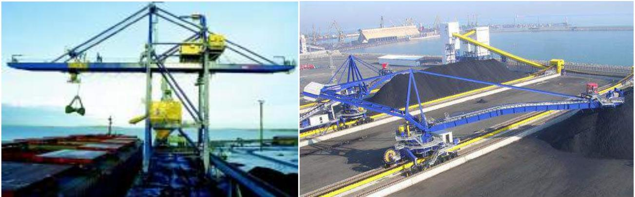
Figure 143: Some examples of coal terminal equipment. Gantry crane (left) and stacker/reclaimer (right)
