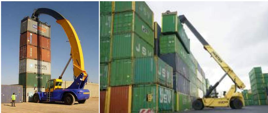
Figure 141: Two different types of reach stackers (RS)
