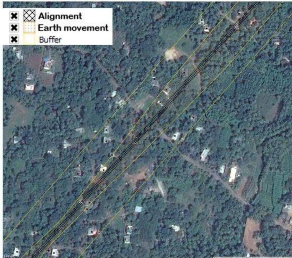
Figure 70: Houses affected within the railway line premises
