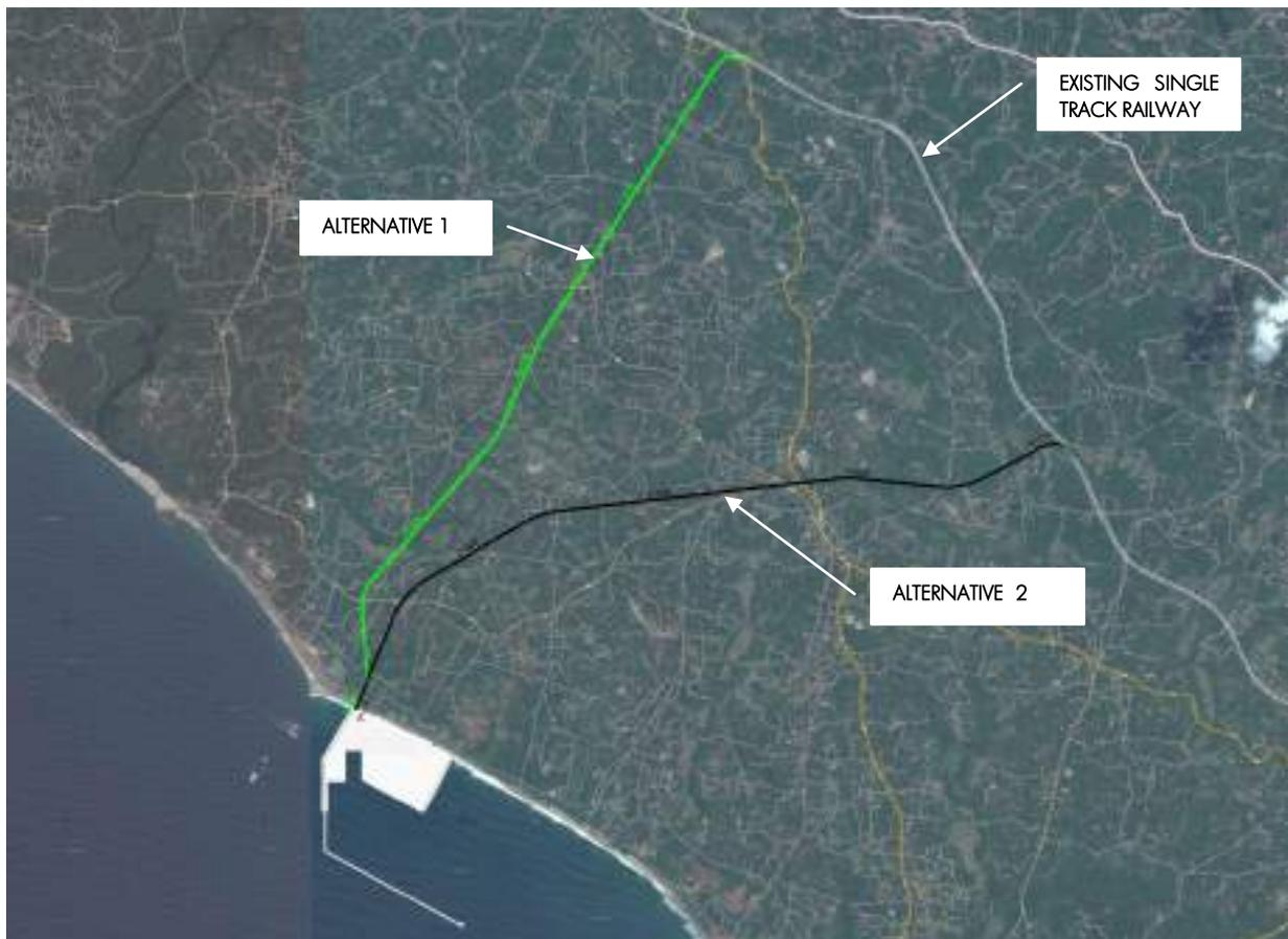
Figure 146: Alternatives 1 (green) and 2 (black) for rail connectivity
