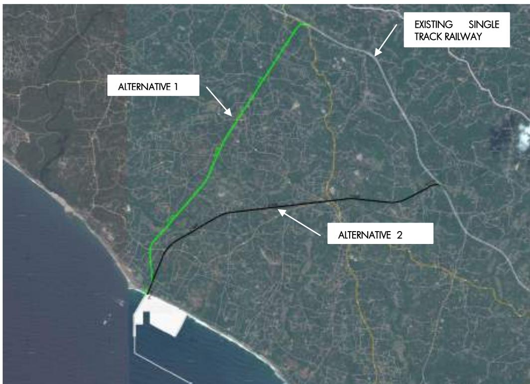
Figure 13. Alternatives 1 (green) and 2 (black) for rail connectivity
