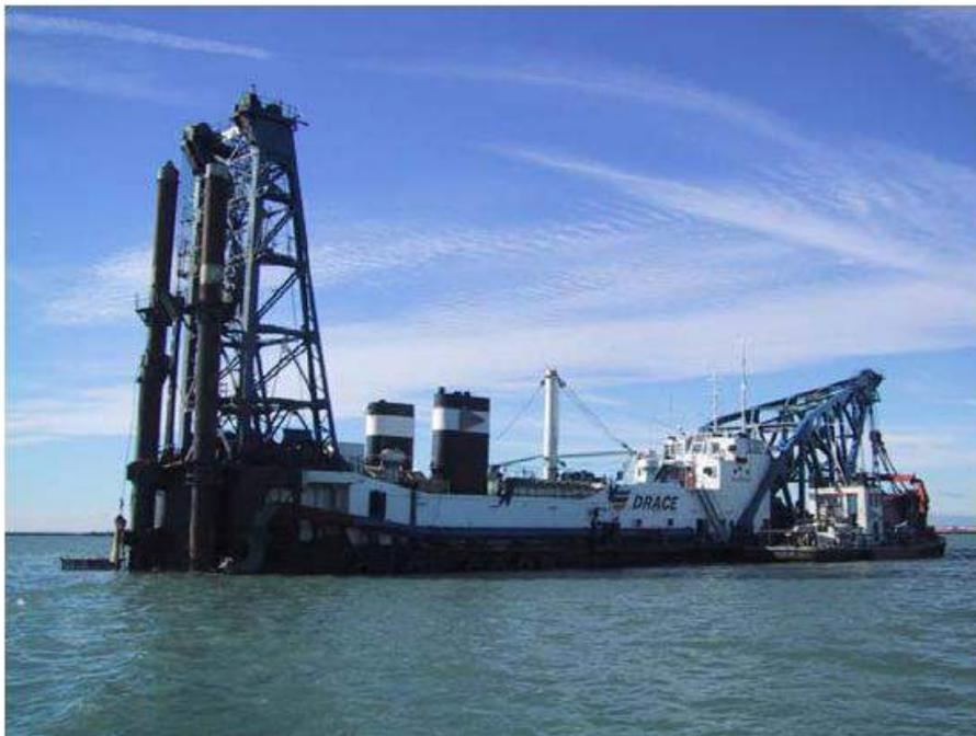
Figure 132: Cutter Suction Dredger
