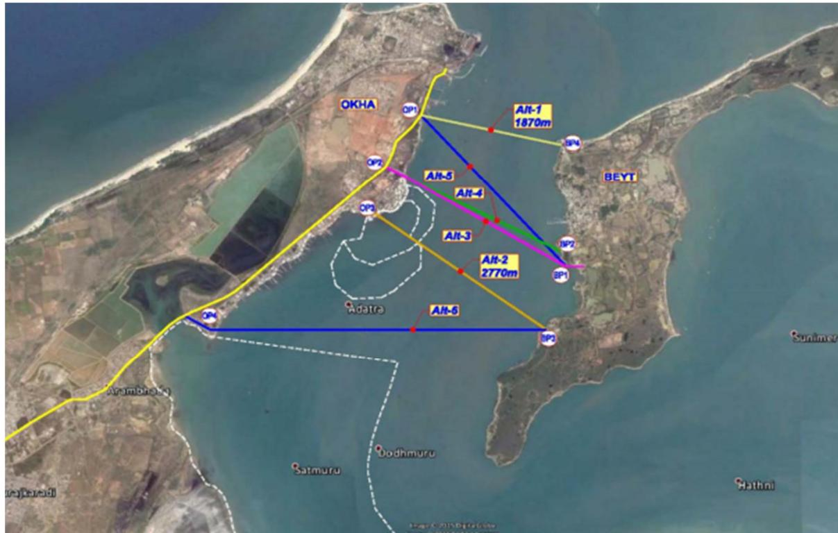
**Figure 3.11 Proposed Alternative Alignments for the Road Bridge**
