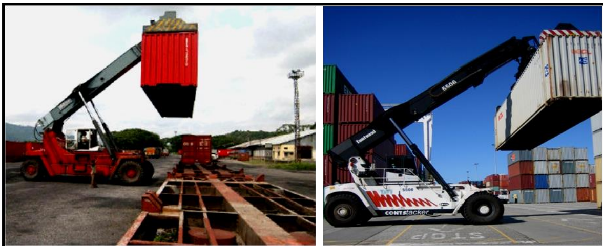
Figure 7.14 Snapshot of Typical Reach Stacker Handling
