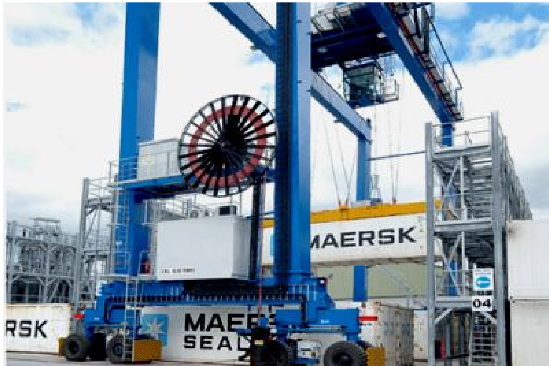
Figure 7.5 Typical E-RTG for Yard Operation
