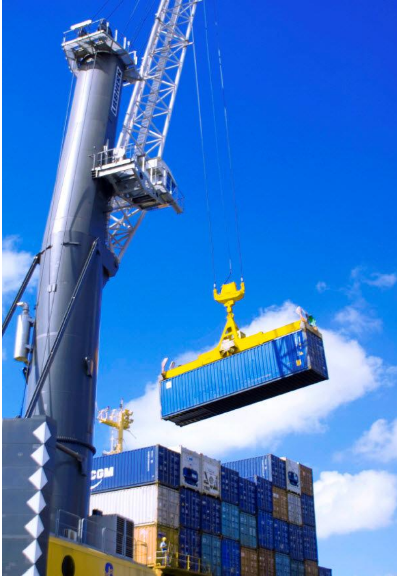
Figure 7.4 Mobile Harbour Crane with Spreader Arrangement
