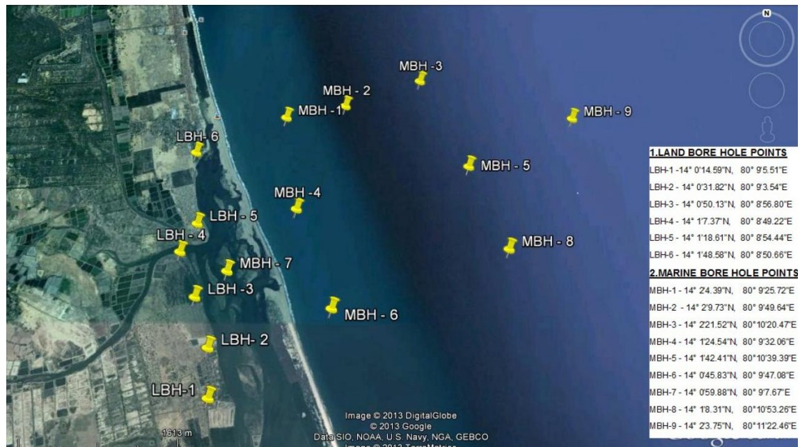
Figure 2.6 Location Plan of Land and Marine Boreholes
