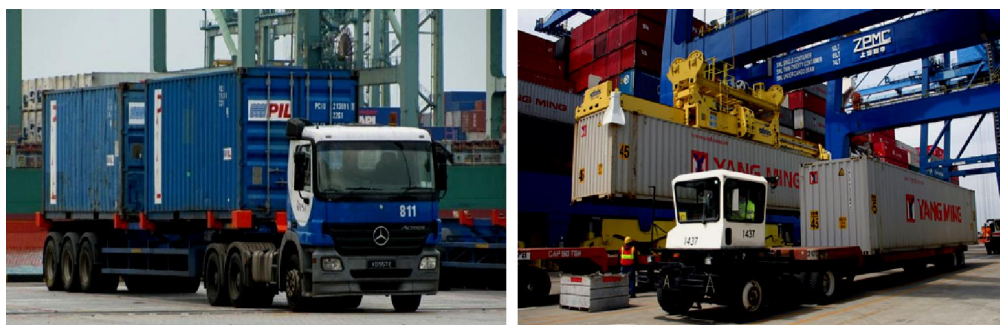
Figure 7.9 Typical ITV for Handling Containers
