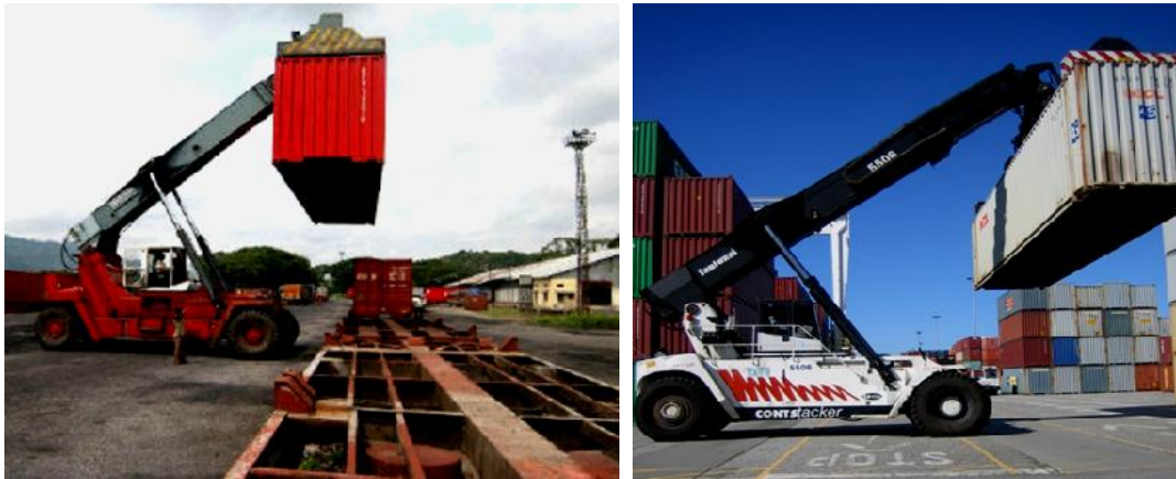
Figure 7.8 Snapshot of Typical Reach Stacker Handling
