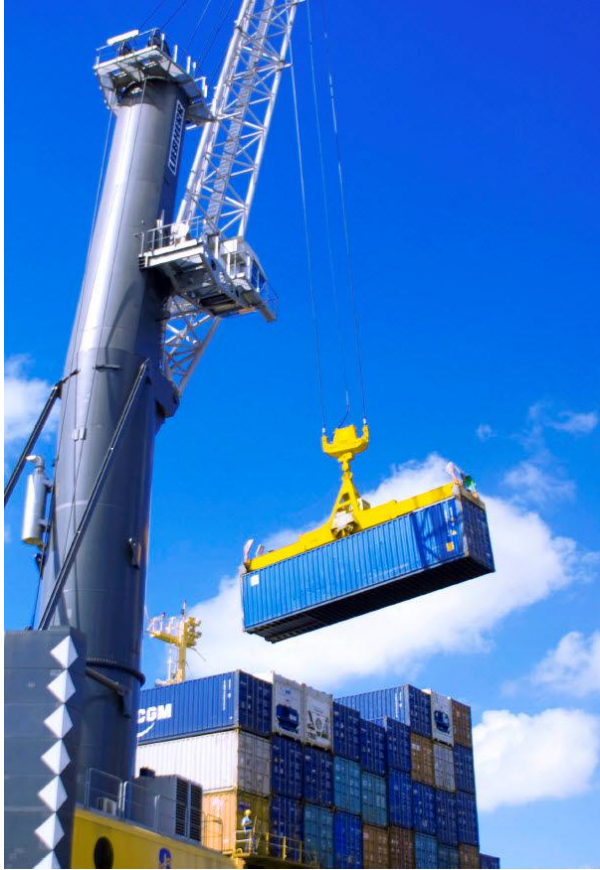
Figure 7.8 Mobile Harbour Crane with Spreader Arrangement
