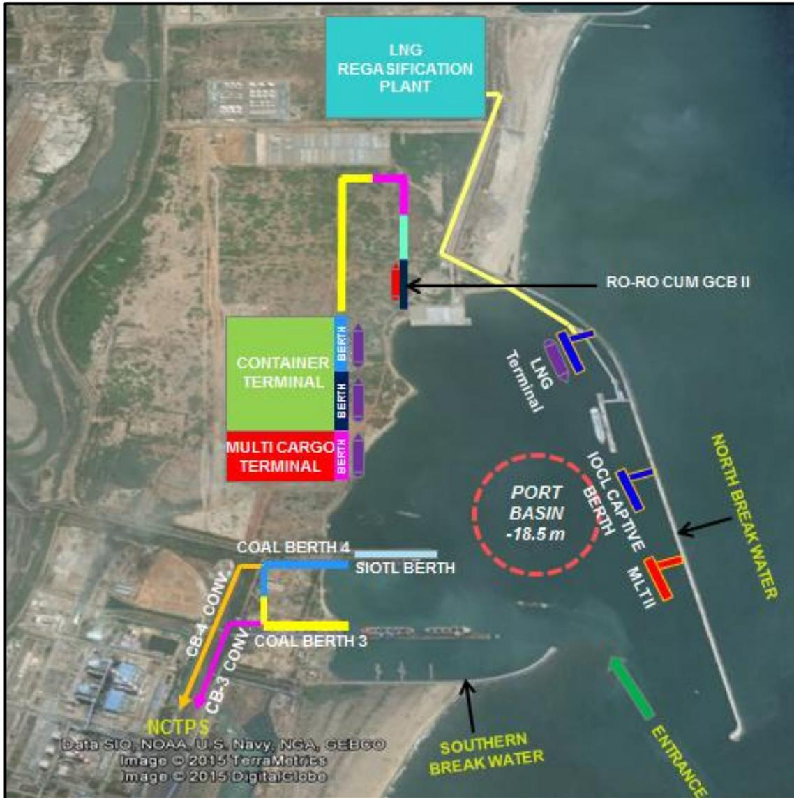
**Figure 10.2** Port Layout with All Facilities Up to 2020
