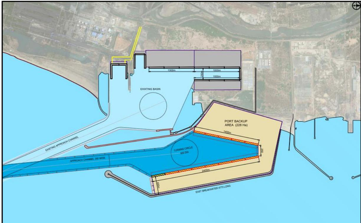
**Figure 9.4** Potential Outer Harbour Development - Alternative Layout 2
