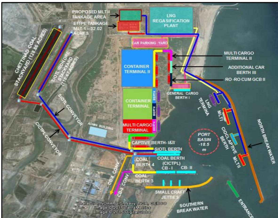
**Figure 10.3** Port Master Plan with All Facilities Up to 2035
